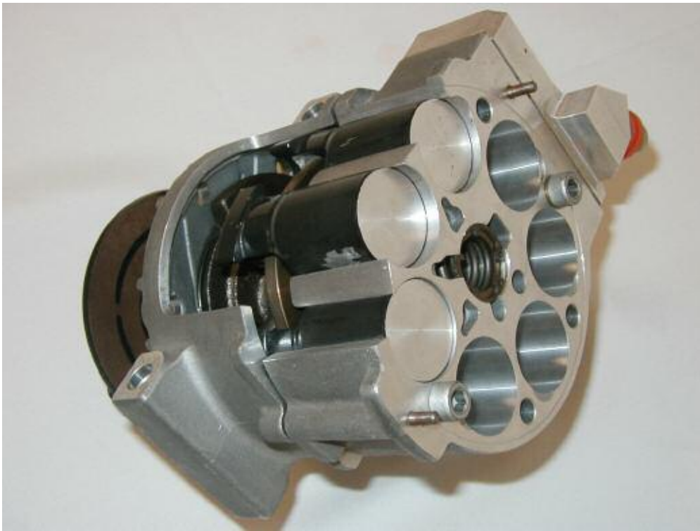
Seven Piston Swash Compressor Cut-away
